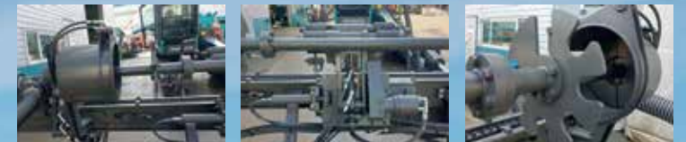
Roller Magazine (ARC) RM Auto rod changer Innovative rod changing system operated by roller & magazine
