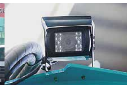
Rear view camera To check an object on the rear side for safety
